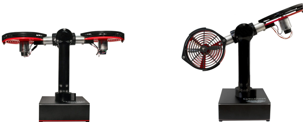
Figure 1: Different configurations of the propellers allowing for different control tasks (Source: Quanser).
